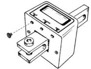
Attach the top hook of the SR 801 Scale to the boom or the lifting strap of the patient lifter. Make sure that the hook is fully engaged, and the safety screw is properly installed.
