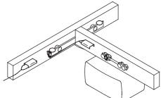
Stick the wire underneath the trolley for traverse rail by means of double sided adhesive tape.
