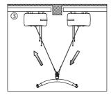
Continue to unroll a little further the lifting strap of the hoist B and then wind up the lifting strap of hoist A.
