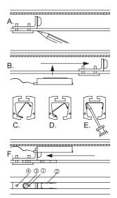
Slide the end stop back to the mark. Unscrew the screw (1) next to the rubber knob of the end stop and fit the spring retainer (2) into the opening of the rail undeneath the end stop. The opening of the spring retainer must face the hoist. The foam rubber disc (3) must be positioned at the bottom end of the spring retainer (4) behind the screw. Tighten the end stop.
